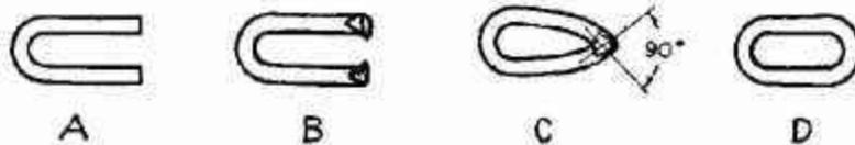
FIG. 269.—Steps in making a link.
